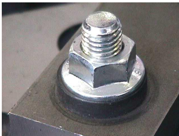
Fig. 31: correct assembly of the vibration dampers;
