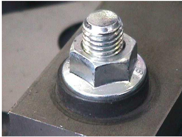
Fig. 33: correct assembly of the vibration dampers;
