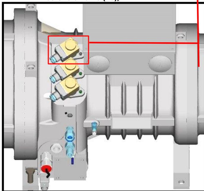
To convert the compressor lay-out from the stepped "L4" to the stepless "LZ" capacity control configuration, replace the plate code 519422 with the plate code 519423. Vice-versa you will perform the opposite switch.
