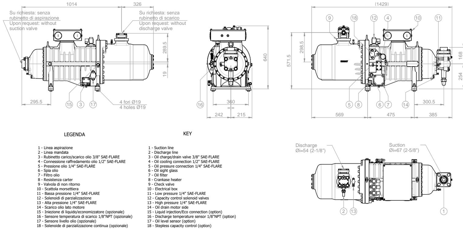
Fig. 44: dimensional drawing of the models: PS3-H070/H080 (drawing code: MSI014)
