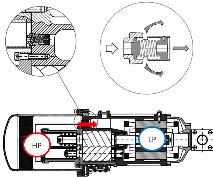
Fig. 30: safety valve shape and position
