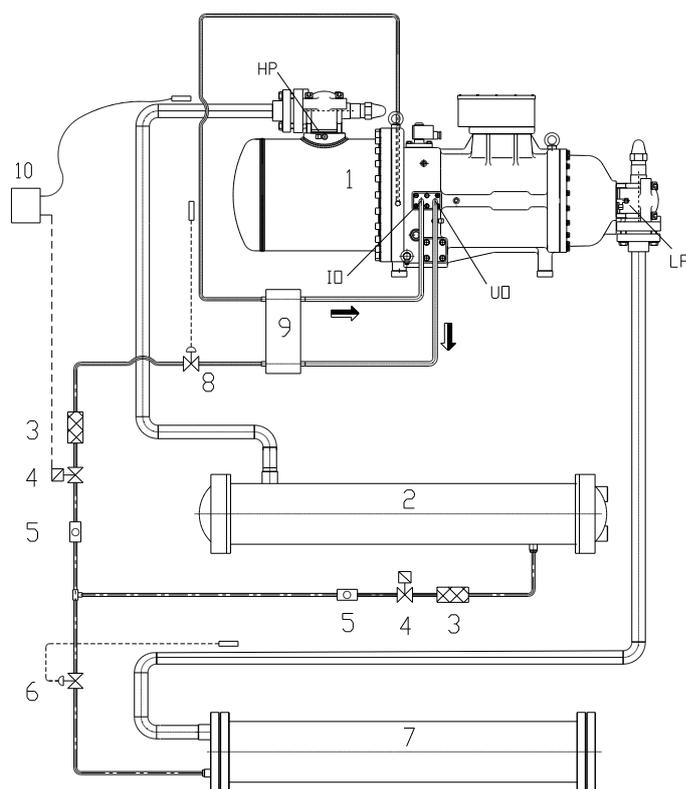
Fig. 56: oil cooling with oil/refrigerant fluid heat exchanger;
