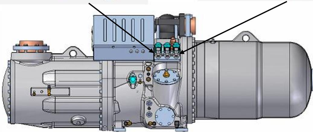
To convert the compressor lay-out from the stepped "L4" to the stepless "LZ" capacity control configuration, replace the plate code 592833 with the plate code 592832. Vice-versa you will perform the opposite switch.
