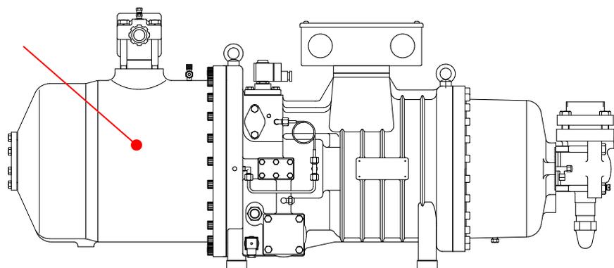
Fig. 10: specific position of the oil separator both for the PS3 series;
