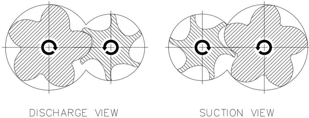
Fig. 6: view of the rotors and correct direction of rotation;
