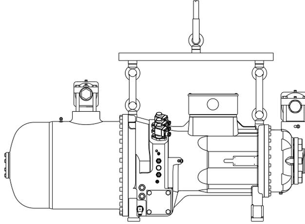
Fig. 50: anchor points for lifting the compressor;
