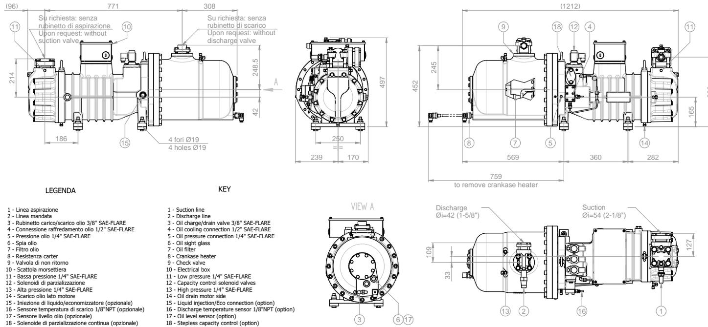
Fig. 43: dimensional drawing of the models: PS3-H040/H050/H060 (drawing code: MSI007);
