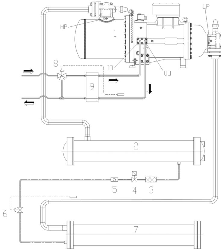
Fig. 55: oil cooling with oil/water heat exchanger
