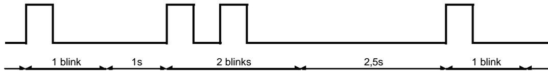
2. "Monitoring Phase" alarm caused by wrong phase sequence.
