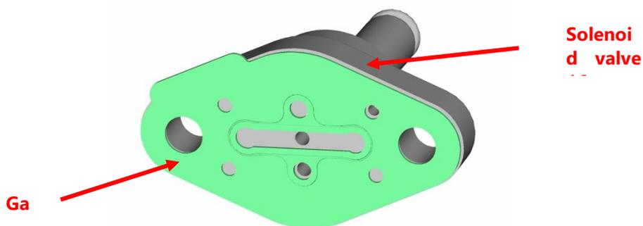
3. In the position 19 fit the cover flange, after inserting the gasket -code 592732- included in the conversion kit;
