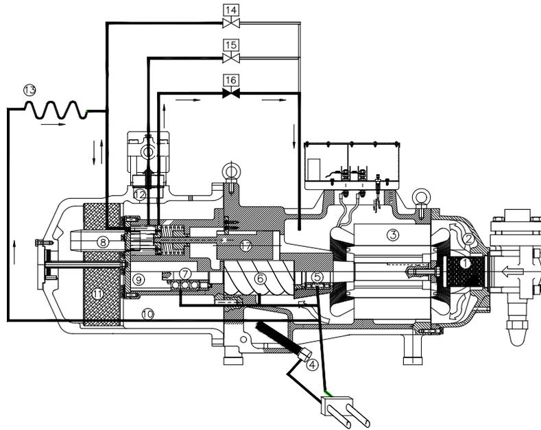
Fig. 22: capacity control at 75% step;
