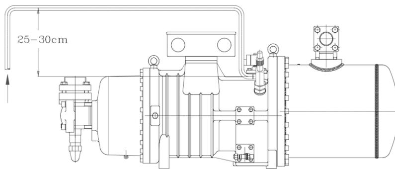
Fig. 54: layout of the liquid injection line;
