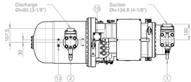
Fig. 47: dimensional drawing of the models: PS3-H200/H220/H240 (drawing code: MSI025)
