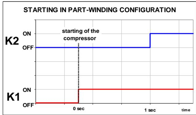
Fig. 39: connection diagrams to the three-phase network and time charts for the activation of contactors K1,K2 and K3 in the two compressor starting modes: star-delta and part-winding;
