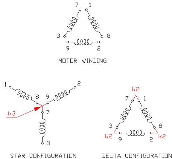
Fig. 38: internal winding connections for the motors with star-delta configuration
