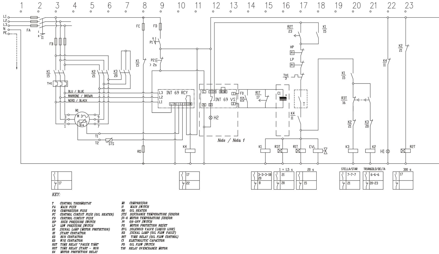
Fig. 36: wiring diagram for the connection of the flow switch; electric motor with star-delta configuration YΔ (MCE008\$2);
