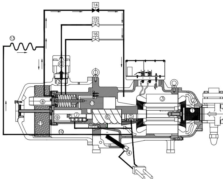
Fig. 20: Minimum capacity control oil circuit
