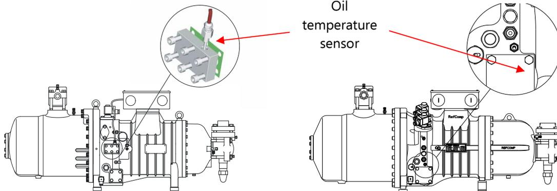
Fig. 41: position on compressor for oil temperature monitoring sensor
