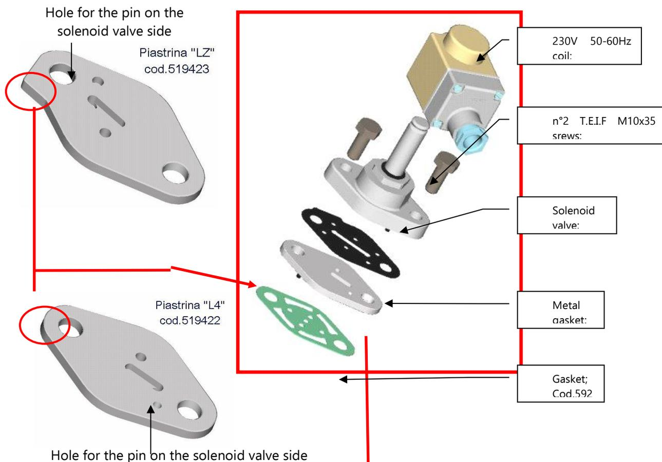
**Position of the plate: underneath the solenoid valve (16);**
