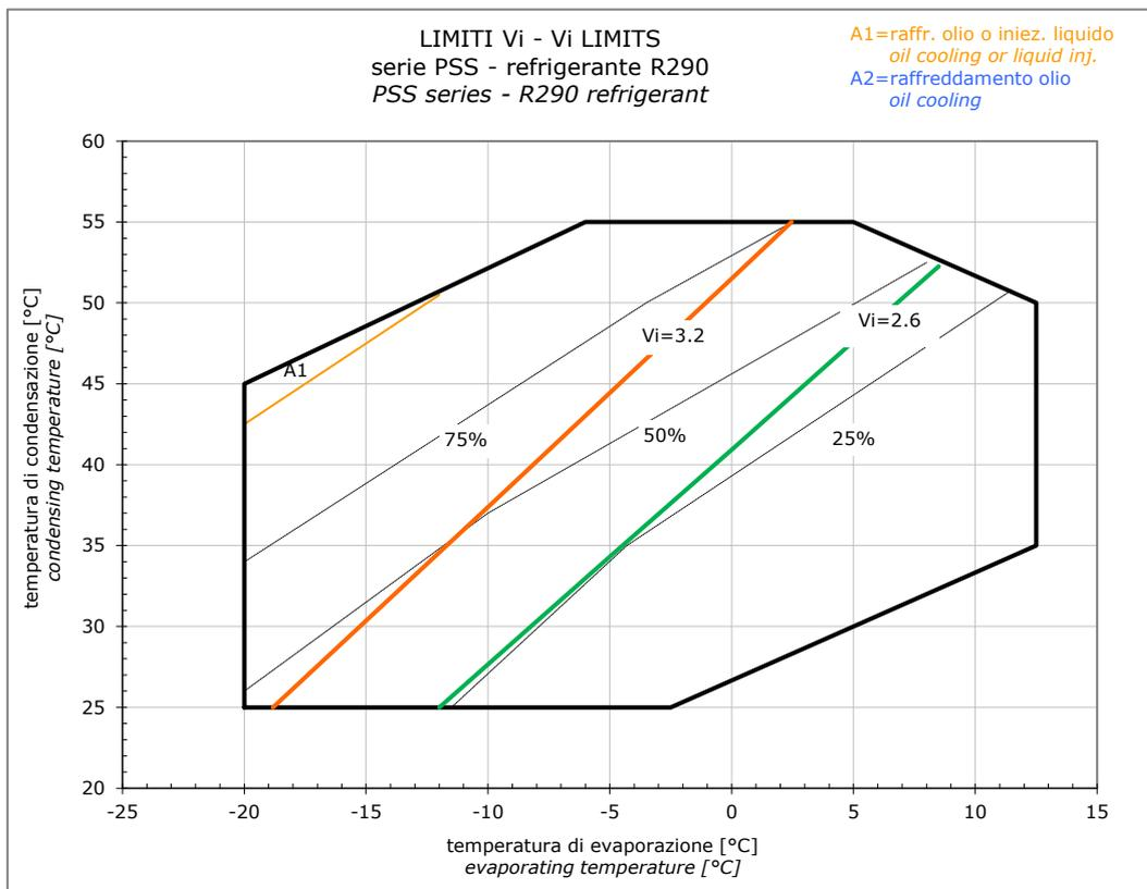
Fig. 8:  $V_i$  values recommended with R290
