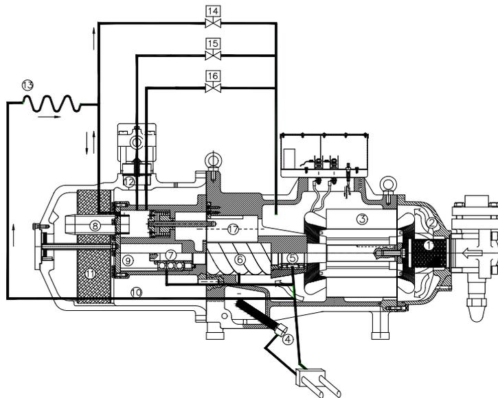
Fig. 23: capacity control at 100% step
