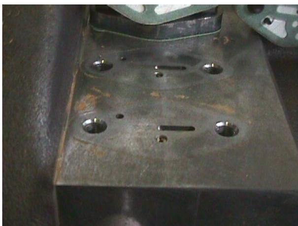
5. Replace the solenoid valves 14 and 15 in their original position, after inserting the gaskets -code 592731;
