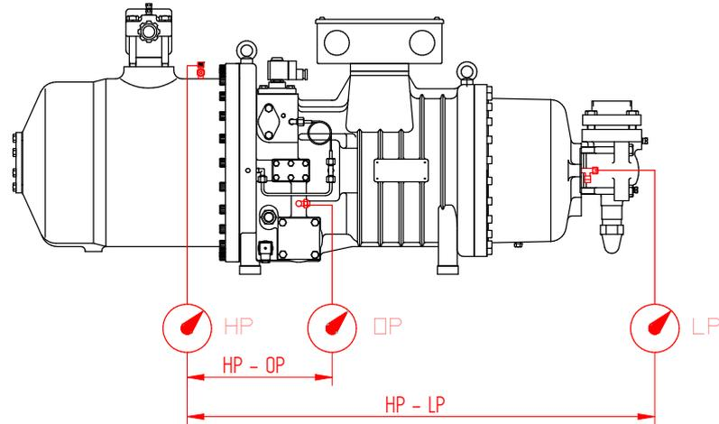
Fig. 17: measuring the HP, OP and LP pressure values in the PS3 series
