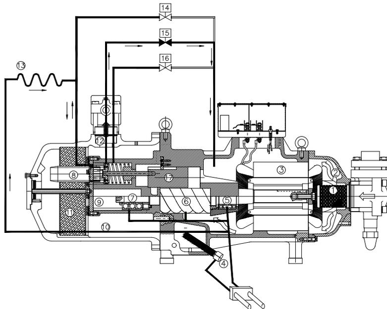
Fig. 21: capacity control at 50% step
