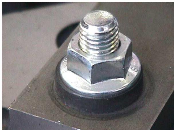
Fig. 33: correct assembly of the vibration dampers;
