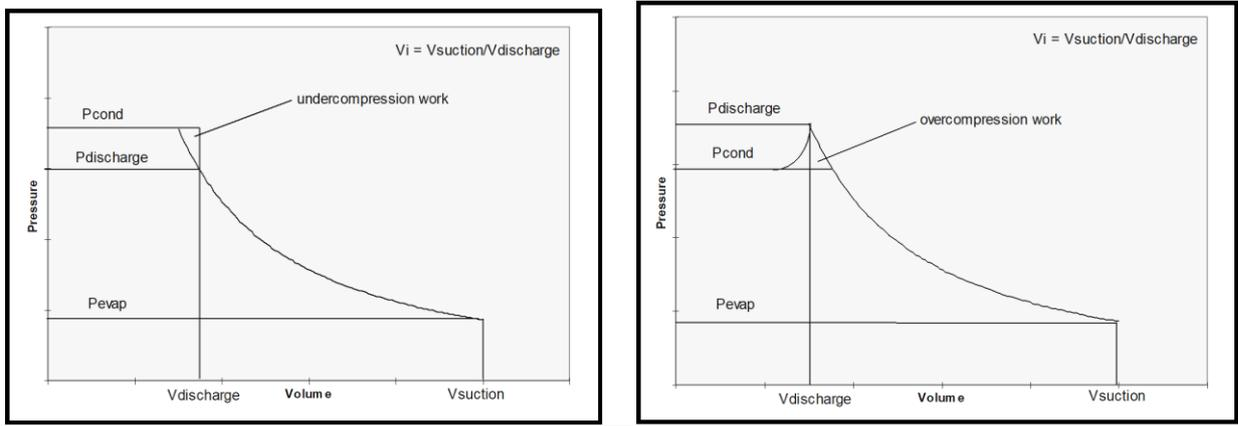
Fig. 7: the compression process on the p-V diagram;
