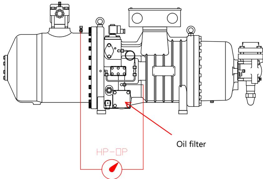
Fig. 12: position of the oil filter in the PS3 series compressors (in models H040/H050/H060 the filter is located inside the oil separator) and definition of the HP-OP pressure drop across the filter;
