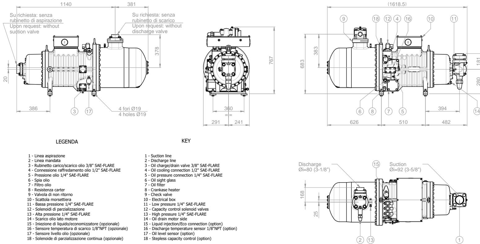
Fig. 46: dimensional drawing of the models: PS3-H140/H160/H180 (drawing code: MSI001)
