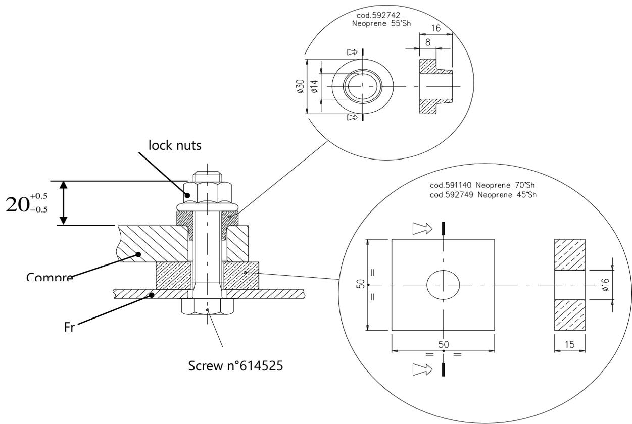
Fig. 34: assembly diagram for the rubber vibration
