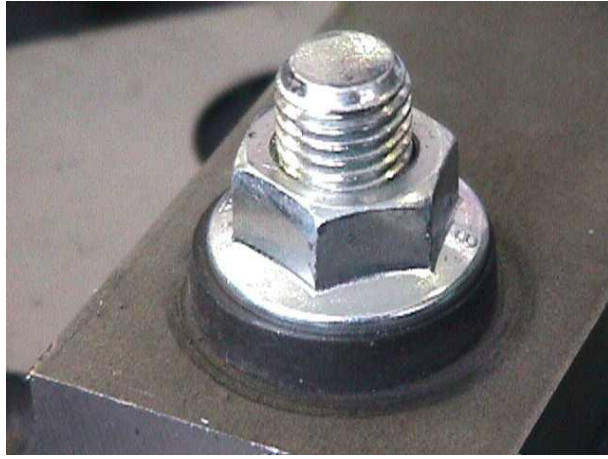
Fig. 31: correct assembly of the vibration dampers;
