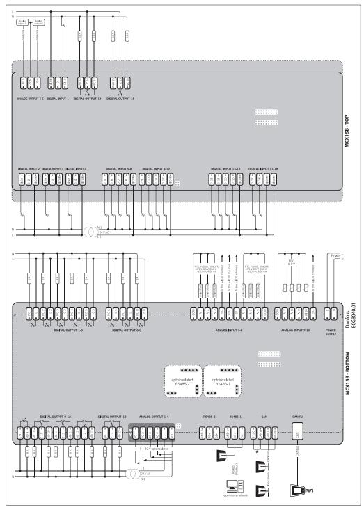
\*NOTE: connection has to be made on the first and last local network units, make the connection as close as possible to the connector \*\*NOTE: optoinsulated analog outputs voltages are referenced to contact N1
